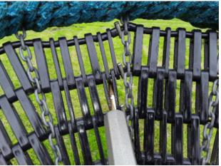
The openings between the slots in the Basket Action: Seat form finger entrapments, when the seat Finding:
