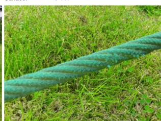
The bottom rope is showing slight damage, and signs of wear Finding:
